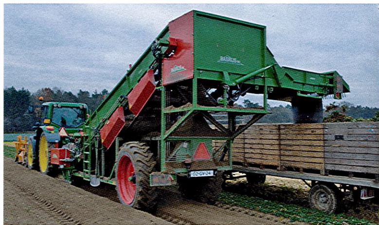
Lifting one bed at a time, the company operates two Dutch-made Basrijs harvesters.
